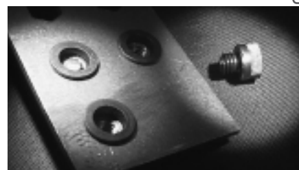
Destructive test, Class 12.9 M8 screw fails at max torque before the thread in high strength Hexsert® inserts
